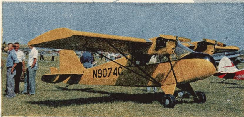
Two 65-hp engines give Irv Miller's "Twin" exceptionally good flight characteristics. Cost to build: \$850.
