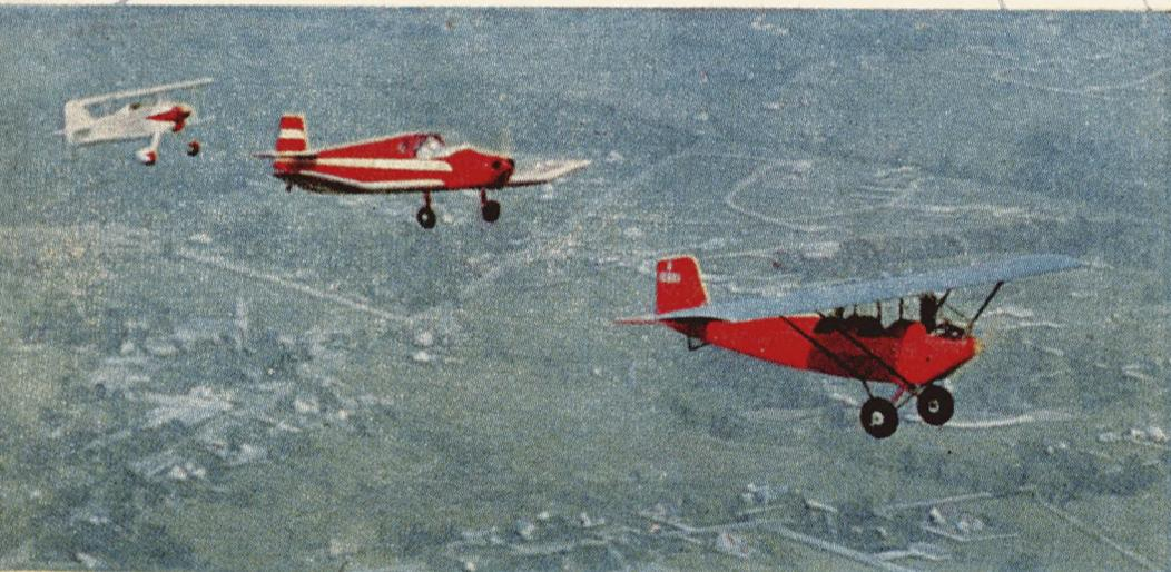
Lead plane is restored Pietenpol "Air Camper," 1930 model, powered by Ford Model-A engine.
