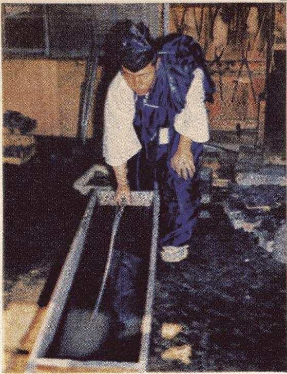
Critical moment comes when blade is doused in water of exact temperature.
