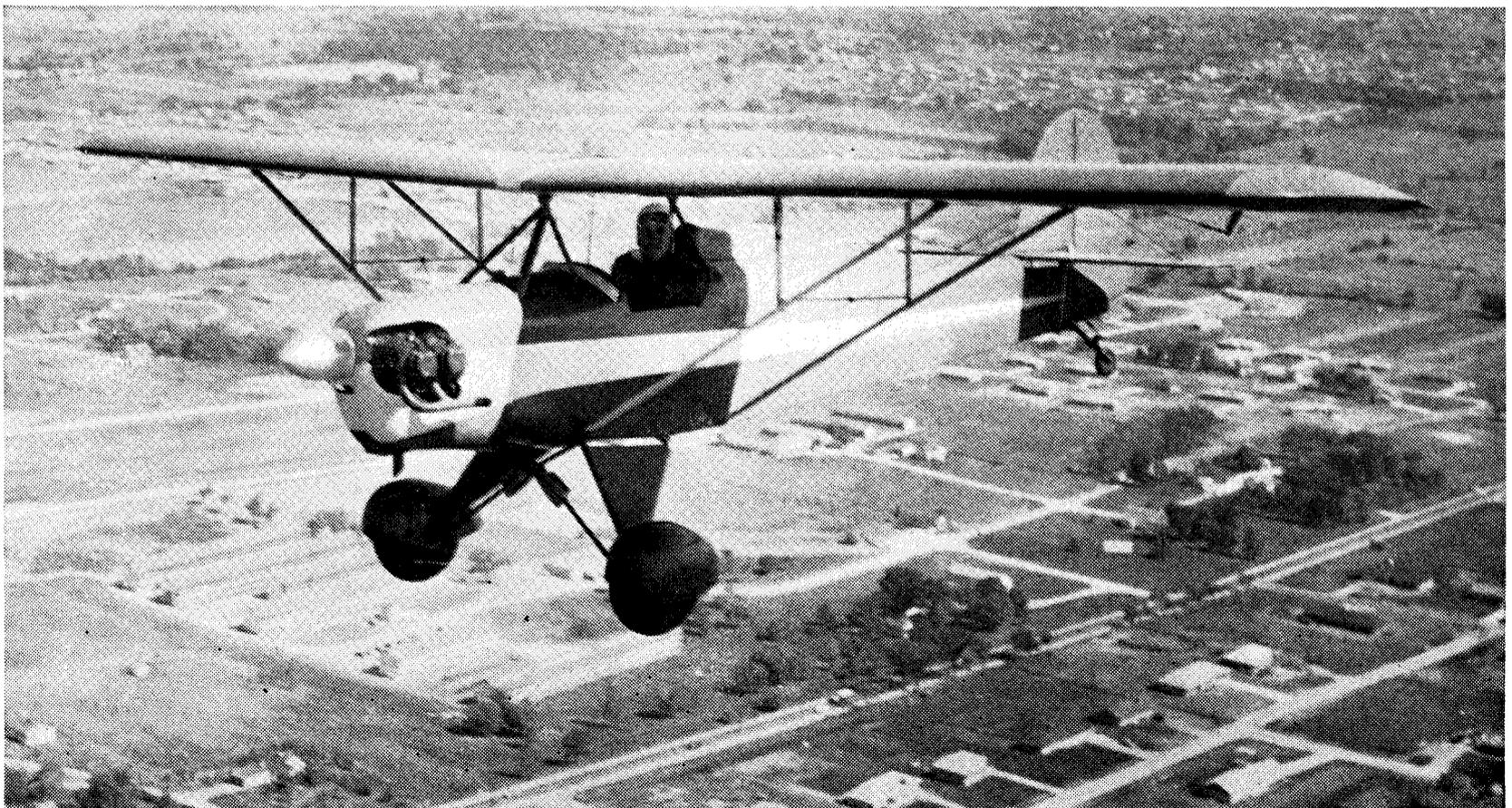
Here Poberezny flies the Baby Ace he built. This plane cruises at 95 mph, can take off in a space of 150 feet.
