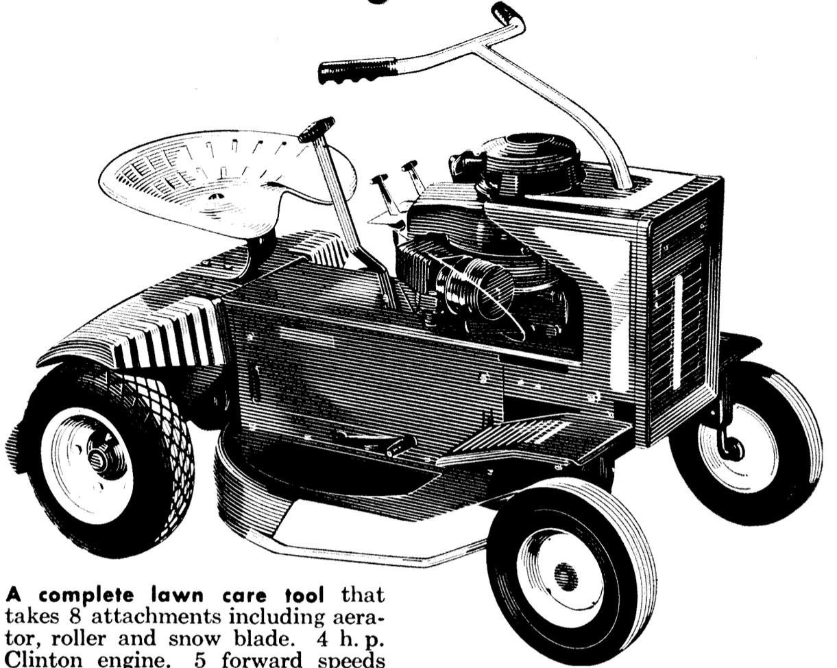
A complete lawn care tool that takes 8 attachments including aerator, roller and snow blade. 4 h. p. Clinton engine. 5 forward speeds plus reverse. Gear drive. Automatic recoil starter. Foot brake. 24-inch suction-lift blade. The side exhaust
